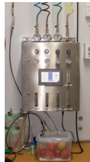
Ultra-low oxygen mixing box – designed by Dr Renate Smit, in collaboration with Josh Kreft of Gas At Site.
